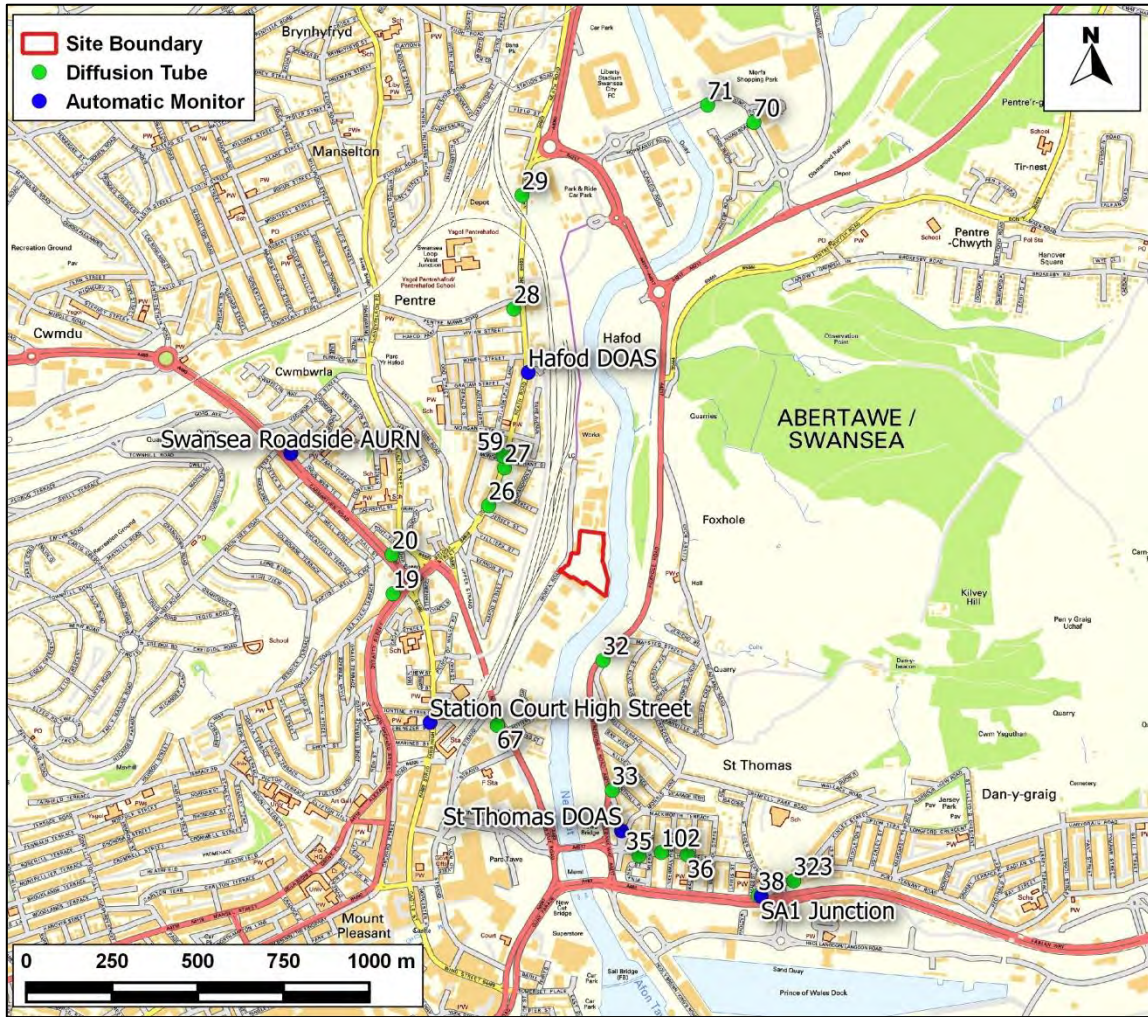
Figure 3: Monitoring Locations (DOAS monitor locations are shown as the location of the transmitter)
